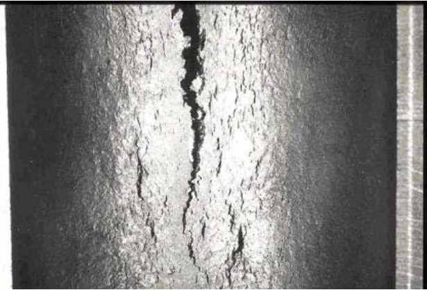
Creep rupture of an HK40 heater tube
