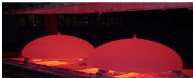
Figure 6. Stress relief process (image courtesy of Myungjin Heat-Treatment, Inc., www.mhti.co.kr ). [Color figure can be viewed at wileyonlinelibrary.com ]
