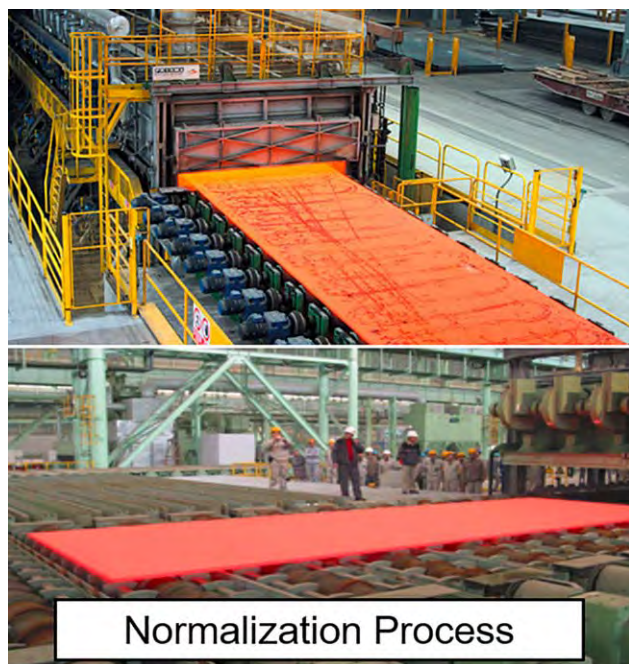
Figure 4. Normalization process (image courtesy of Prisma Impianti, www.prismagroup.it and Wesman Group, www.wesman.com ). [Color figure can be viewed at wileyonlinelibrary.com ]
